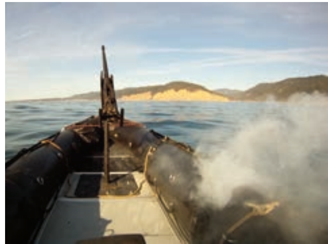
(Left) Lockheed's prototype 10 kW Area Defense Anti-Munitions (ADAM) laser system is a transportable ground-based fiber laser system. (Center) In a test, the ADAM laser system destroyed 11 small-caliber rocket targets at a range of 2 km. (Right) In May 2014, the first maritime tests of the prototype ADAM laser system burned a hole through the rubber hull of a boat moving in the ocean. Lockheed Martin
