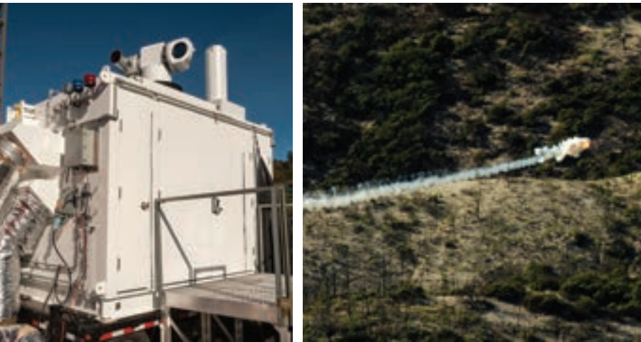
(Left) Lockheed's prototype 10 kW Area Defense Anti-Munitions (ADAM) laser system is a transportable ground-based fiber laser system. (Center) In a test, the ADAM laser system destroyed 11 small-caliber rocket targets at a range of 2 km. (Right) In May 2014, the first maritime tests of the prototype ADAM laser system burned a hole through the rubber hull of a boat moving in the ocean. Lockheed Martin
