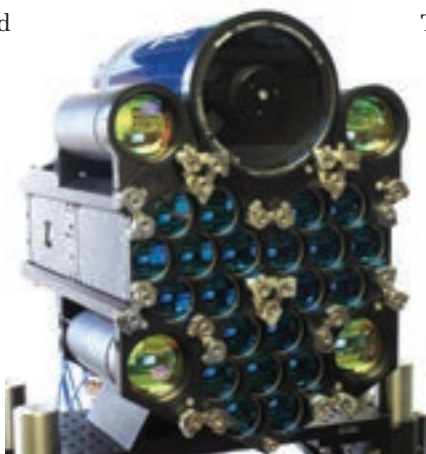
DARPA and partner Optonicus designed this optical phased array used in the Excalibur demonstration to improve laser weapons performance. Optonicus
